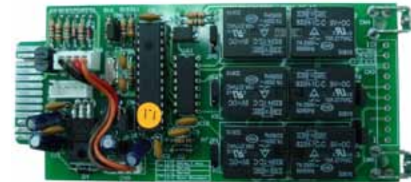
True Relay Contact Board (DCE-B card)
