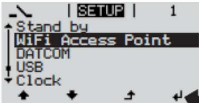
Fig.1: Inverter display Setup menu
